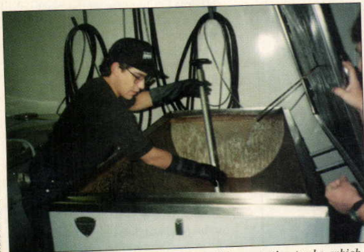
Jim Dallarosa cleans one of the original fermentation tanks, which were converted from dairy equipment.
