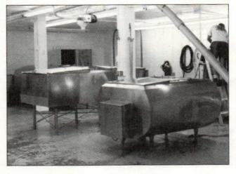
Most of the equipment is made from reconditioned dairy tanks, including this mash tun. left, and open fermenter, right.
