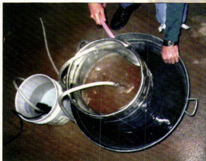
Using an immersion chiller with an ice bath speeds up the cooling process.
