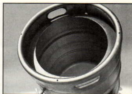
First release any residual pressure in the keg (careful; it can be dangerous). Then cut the top off, sizing the hole slightly smaller than your lid.
