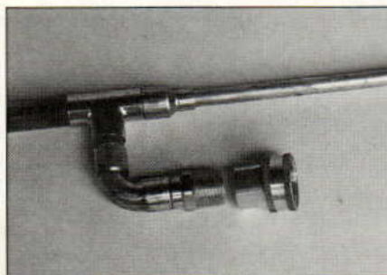
Here is a "dry fit" of all parts including a male straight pipe and the very important garden hose adapter.
