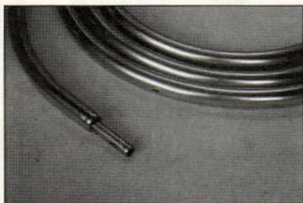
A tube within a tube: The 1/4-inch inside diameter copper tubing inside the 5/8-inch inside diameter tubing.
