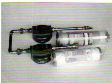
Here's how the plumbing goes together. The lower filter is the carbon block.
