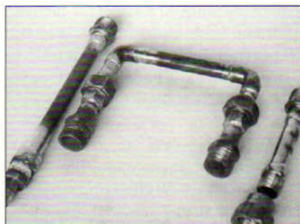
Fully assembled plumbing parts: Inlet pipe, outlet pipe and two connections.
