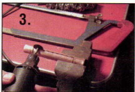
The author uses a Dremel tool cut-off wheel for cutting his tube lengthwise.
