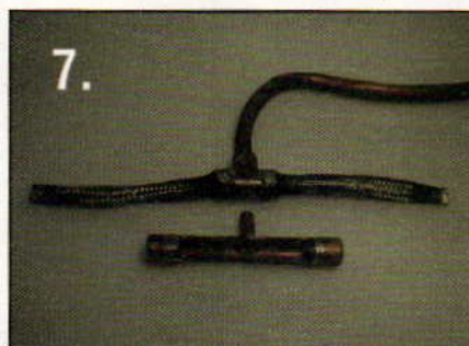
Two prototype kettle filters, both easy to sanitize in boiling water or the oven.
