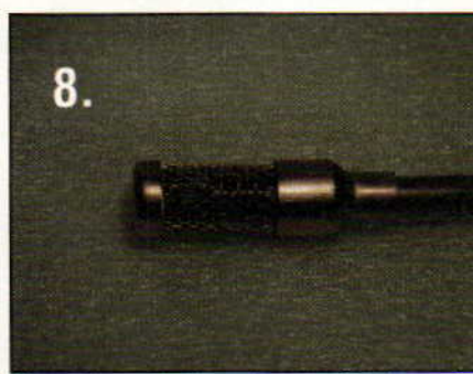
The adapter is bored out to fit the racking cane. Note cane inside the screen.
