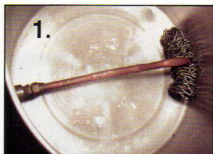
If you have a spigot, an easy solution is a bent tube and a stainless sponge.
