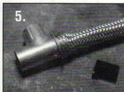
Woven stainless-steel sheathing was forced over this copper "T" connector.
