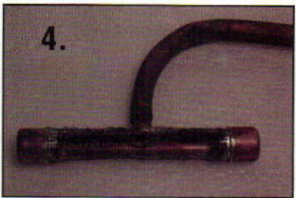
For the final step, wrap a screen around the tube and then solder it.
