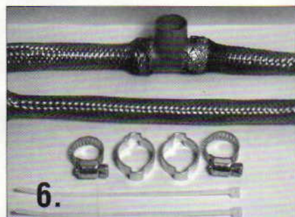
The best solution to hold the sheathing is to use stainless-steel crimp clamps.
