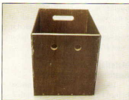
To add handles for easier transport: Just start with two drilled holes, then connect the dots with a saber saw.
