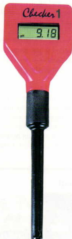
A handheld pH meter. When used properly, a pH meter is easy to use and more accurate than pH test papers.
