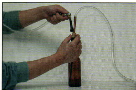
CP filler: The beer flows from the keg's tap through the copper tube; the CO 2 comes from the keg's tank through a tire chuck, valve and sport-ball needle.
