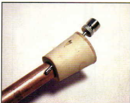
You also push the needle through the hole you drilled in the stopper.
