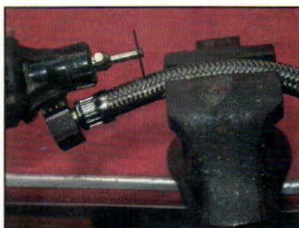
I used a Dremel tool to cut the flex from its fittings. Look for a sturdy weave.
