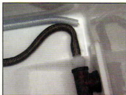
This is the way the handy stainless flex slips onto the Kynar fittings.
