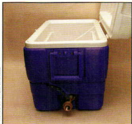
This handy 12-gallon cooler holds 25 pounds of grain during the mash.
