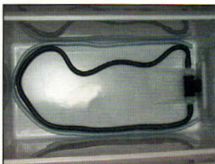
The plastic tube from inside the flex will help keep the flex in place.
