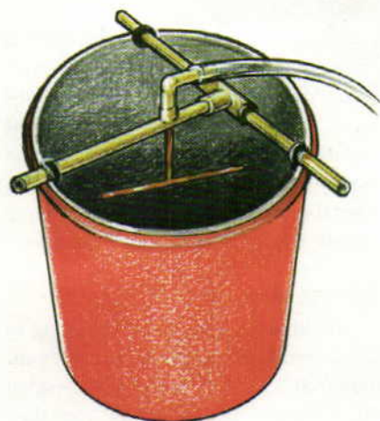
A sparge arm is like a little sprinkler that sprays water over the mash.
