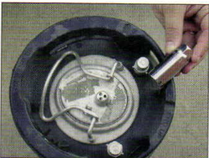
To remove pin-lock fittings, you need a modified 1 1/16-inch deep socket.
