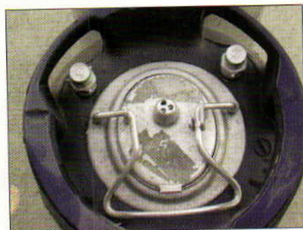
The pin-lock beverage keg uses pins and a twist-on locking system.
