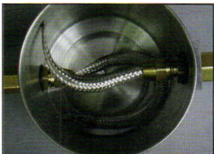
A closer view of your finished hopback with my favorite stainless sheathing.
