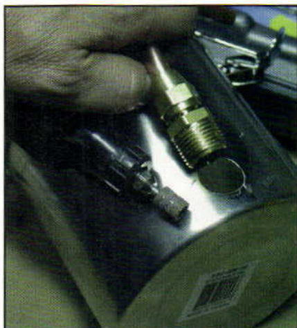
Drill a starter hole and then enlarge it progressively until it fits.
