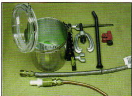
The parts: fittings, a tubing cutter, tubing bender, flare tools and hose.
