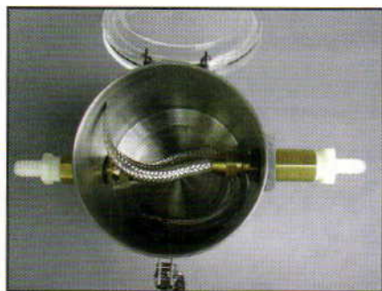
The final product: Note the bulkhead fittings for both the inlet and outlet.
