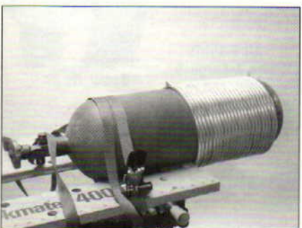
Forming a coil is easy: Just loop the copper around a carbon-dioxide tank.
