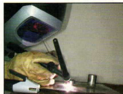
TIG is similar to oxy-acetylene welding or brazing; there's a torch head that emits gas, argon in this case, and heat is created by an electric arc.
