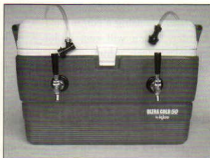
The finished jockey box (exterior view), complete with two tap handles.
