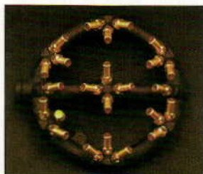
Left: A ring burner is a cast-iron circle with holes in concentric rings around the burner. It has an adjustable air inlet and runs better at lower pressures. Center: This is a multi-jet natural gas burner. Each jet has an orifice and four air-inlet holes. They are quiet and put out more heat than other standard burners. Right: A high-pressure burner is two pieces held together with a bolt. It has an adjustable air inlet and lots of power for big boils.
