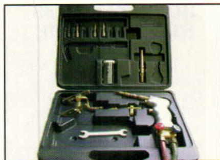
This is the author's Henrob 2000 oxy-acetylene torch set. He's used it to weld mild steel and aluminum, braze and cut mild steel, and braze stainless.
