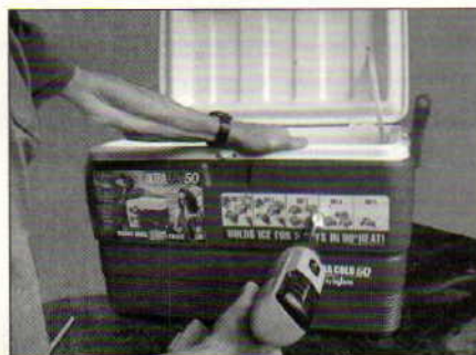
Measure the height and left-right distance to evenly place your spigots.
