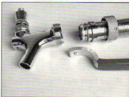
Use a faucet wrench to fasten the knurled collar of the shank to the tap.
