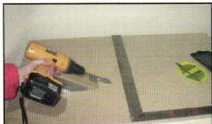
Drilling holes at a consistent angle can be done with a homemade angle-guide made from a cardboard box.
