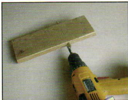
The shutoff mechanism for our bottle sanitizer pivots at a point that is off-center. The board pivots on dowels.
