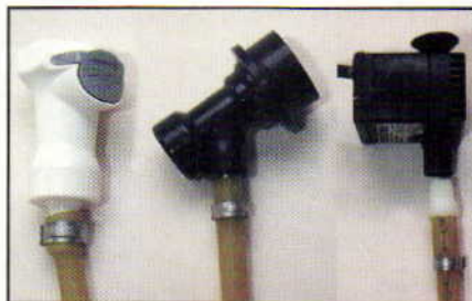
Our device can attach with a CPC quick-connect, a ball-lock keg connector or a connection for a RIMS pump.
