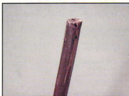
The holes in our wand tip were made with a small drill bit. Sand the copper around the holes when finished.
