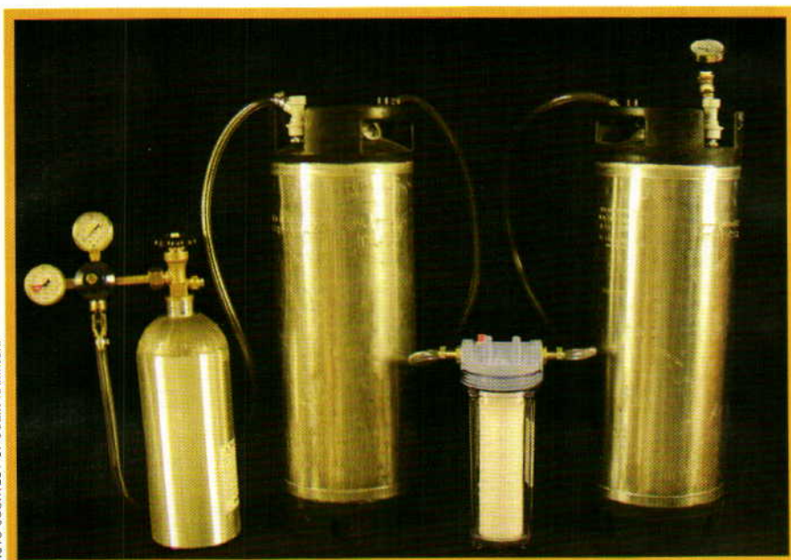
Here is a set-up for filtering carbonated beer. Gas flows in the "gas-in" fitting on the keg to be filtered (at left). This pushes the beer out the "out" fitting, through the cartridge filter and in the "out" fitting (so the beer enters the receiving keg, at right, from the bottom). There is a pressure-relief fitting with a gauge on the "gas-in" fitting on the receiving keg. The pressure gauge on the receiving keg must read higher than the serving pressure for the beer: 30 psi in and 14 psi out works well.
