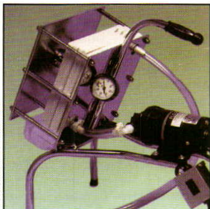
This is a pad filter. They are commonly used by home winemakers and work just as well for filtering beer.
