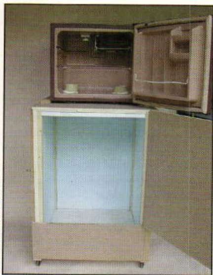
The DraftErator is an insulated box cooled by a dorm fridge. It will keep four Cornelius kegs at serving temperature.
