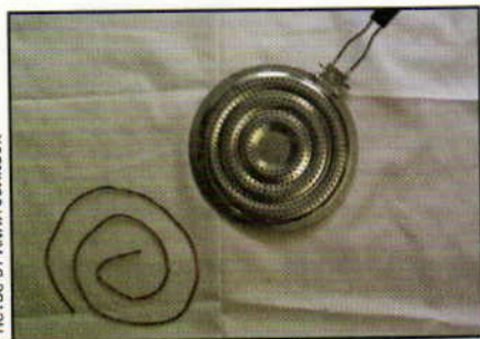
A heat diffuser prevents hot spots on the bottom of your brew pot, reducing the likelihood of wort caramelization.
