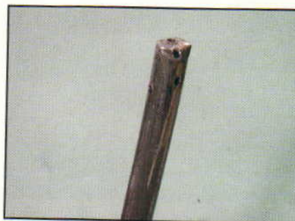
A series of holes in the wand tip directs cleaning fluid to all parts of the carboy.
