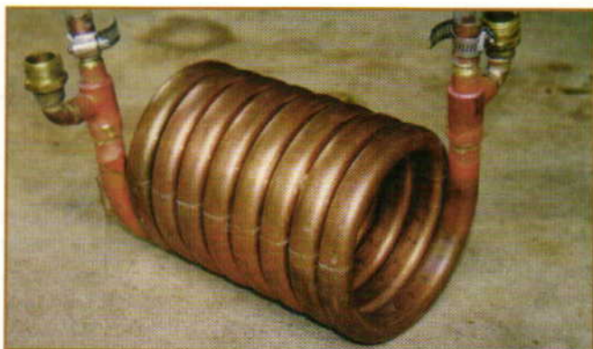
Counter-flow wort chillers are more difficult to clean than immersion chillers, but they can cool your wort more quickly. Cold water runs through the outer tube.
