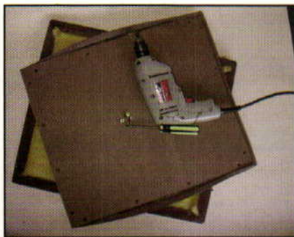
The plastic molding on the refrigerator door is replaced with a panel made of thin masonite.
