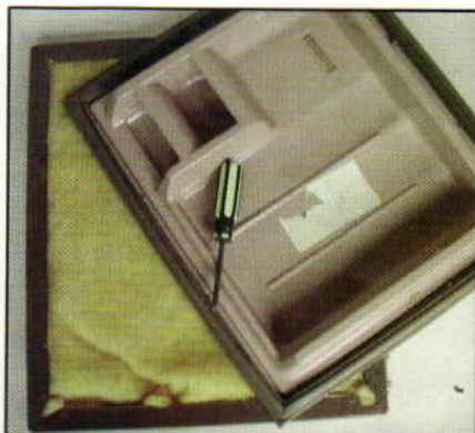
The plastic molding on the refrigerator door must be removed to make room for the water bath and chiller.
