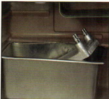
The chiller plate sits in a water bath cooled by the fridge. The bath is made from a stainless steel sink.
