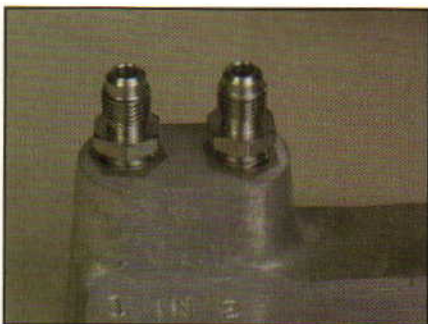
Use Oetiker clamps on all connections, like the flared fittings on this chill plate. This will prevent leaks.
