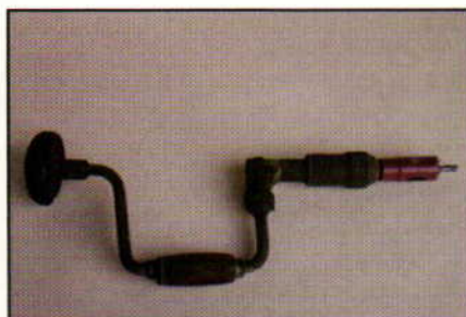
To drill holes through the fridge door and masonite for the tap, I had to chuck my hole saw to a hand drill.
