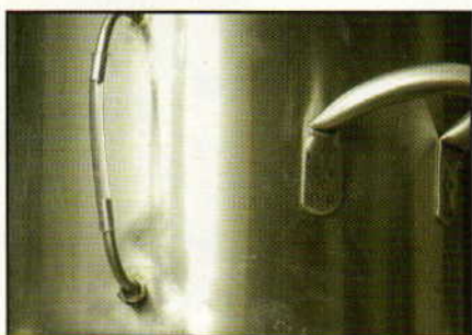
Once the tubes are welded to the kettle, insert the tubing. The final step is to secure the tubing with Oeticker clamps.
