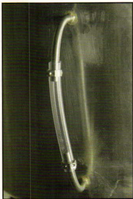
Using simple tubing for illustration, here's how our sight glass will look. The tube is held with Oeticker clamps.
