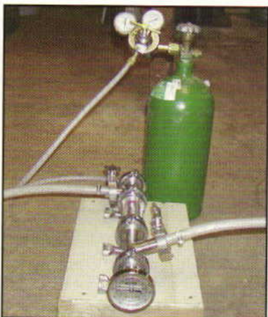
Alan's stainless-steel aerator injects oxygen into the wort at 3 psi.
