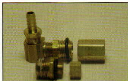
If you don't want to weld, you can make a no-weld sight glass from compression fittings like these.
