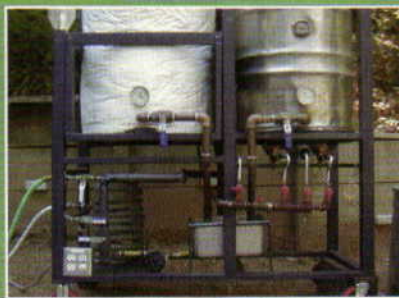
The lower section of the brewery houses the chiller, sump and burners.
