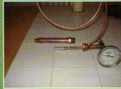
Here's a look at the oxygen injection system, disassembled.
