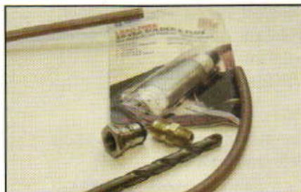
Our cleaner for quick-disconnect (QD) tubes will take a bit of drilling and soldering to make the proper adapter.
