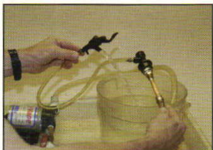
Circulating cleaning solution through this tap powers away the hose residue.
