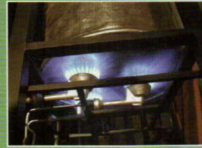
Lift-off! Here are three 150,000-BTU burners being fired under the kettle.
