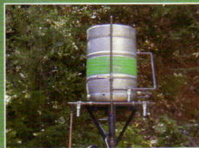
The hot-liquor tank on top can be removed when transporting the rig.
