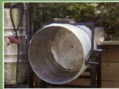
To make cleaning easier, the mash tun can be tipped for dumping out grain.
