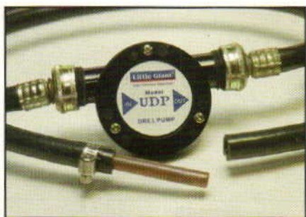
Clamp brewery tubing to the copper tube and then pump cleaning solution through it with our simple CIP device.
