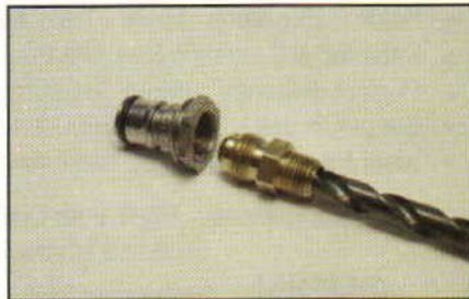
A drilled brass fitting is screwed into a keg-out fitting. The QDs will attach to the keg-out fitting.
