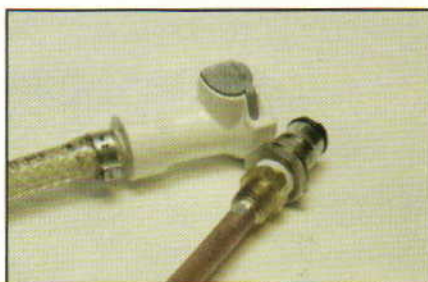
With a copper tube welded to the adapted keg-out fitting, you're ready to clean your quick-disconnect lines.
