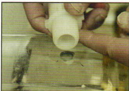
The pilot hole is not large enough to house the spigot. It must be enlarged with another drill bit.
