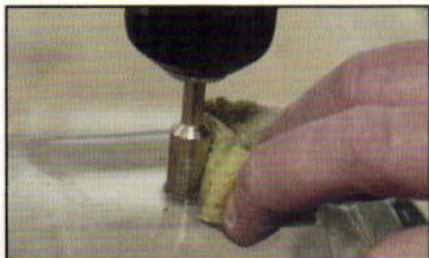
A wet sponge should be used to cool the bit while enlarging the hole. At this stage, the "pool" would not hold water.
