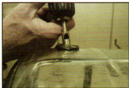
The glass needs to be scored before you attempt to drill the hole. Hold the bit at an angle for this.
