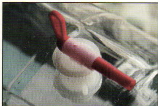
A spigot attached to a carboy can eliminate the need to start a siphon when racking your beer.
