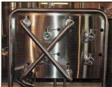
A "divert panel" used for process-pipe cleaning in a closed-loop configuration in the brewery.
