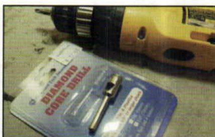
This diamond-tipped drill bit will allow you to drill — slowly — through the thick glass of a carboy.
