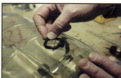
The marked spot is surrounded by a ring of putty that will hold the water that will cool the bit while drilling.
