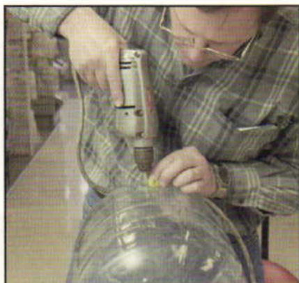
It will take about 30 minutes to enlarge the pilot hole to its final size. Any faster and the glass may crack.
