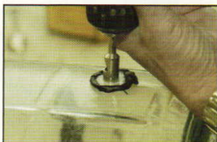
The "swimming pool" around the bit keeps the glass from overheating and, as a result, cracking.
