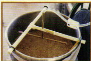
This "whirly-gig" sparge arm is sprinkling the mash with water.
