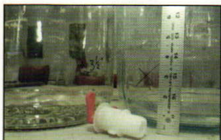
Mark the spot on the carboy where the hole will be drilled. The spigot must be placed above the level of yeast.
