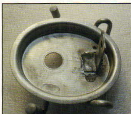
Once the lid hanger is welded to the lid, it will need to be cleaned off.
