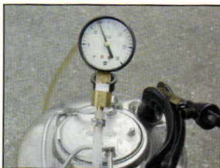
The finished gauge measures the CO 2 pressure on a keg of beer.
