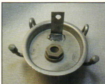
Once the weld is cleaned, the pressure valve can be reinstalled.
