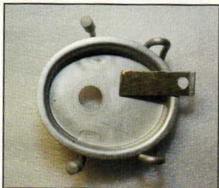
Before welding, remove the pressure-relief valve from the lid.
