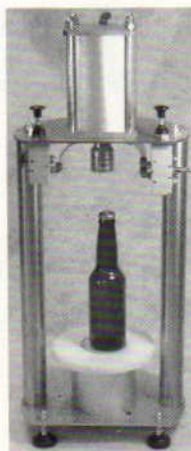
Pneumatic Capper $275 300 bottles/hr
