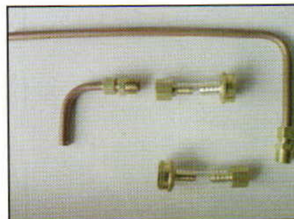
A compression and female barbed connector comprise each bulkhead fitting.
