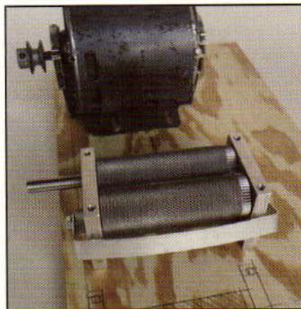
After you decide what motor you are going to use, mount it and your mill.
