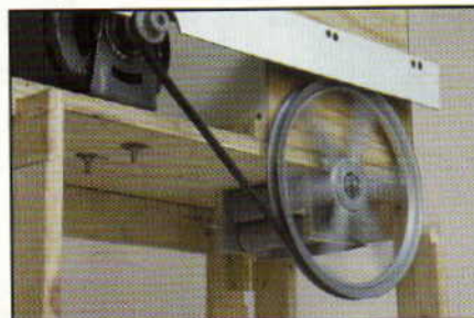
Most AC motors run at 1,750 rpm. The sheaves reduce the rotations on a mill.
