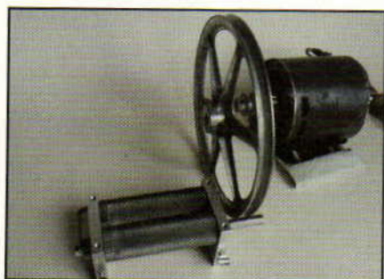
Salvage a 1/2 horsepower motor to power your malt mill.
