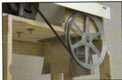
The pulley system slows the motor to an optimum crushing speed.
