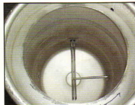
The hot liquor tun with electric temperature probe at the right.
