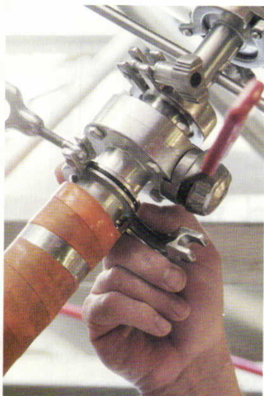
In commercial breweries, pumps move liquid through fixed (immovable) pipes. Frequently, professional brewers use clover fittings to connect their pipes.
