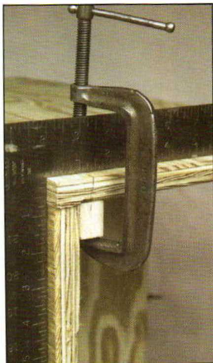
Use a framing square to ensure right angles. Also, be sure to measure edge-to-center distances accurately.
