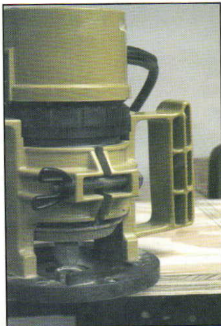
A router can be used to round out the edges of the plywood. A light sanding is also recommended.
