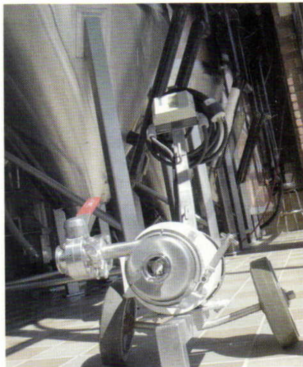
A commercial one-horsepower pump with a center mounted inlet. Unlike with most homebreweries, the vessels and pipes in a commercial brewery never move. This pump is mounted on wheels so it can be moved around the brewhouse and used for different purposes.
