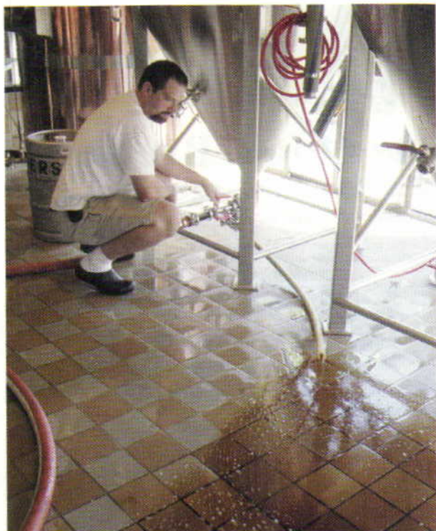
Scott Isham of Harper's Brew Pub and Restaurant transfers a molasses-infused stout into a conical fermenter. A variety of fittings permit him to redirect the flow around the brewery. Here the first bit of wort is spilled into drains until sanitizing fluids have run out of the transfer tube.
