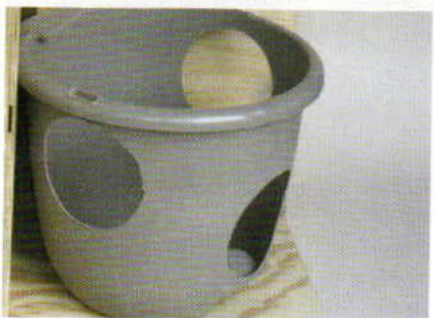
Use a hole saw or saber saw to cut 4" holes in the bucket for ventilation.
