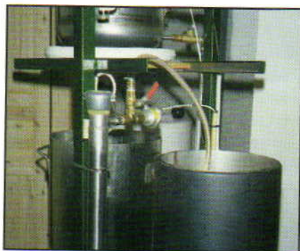
(Top): The counterflow chiller allows Jens' control of his wort temperature. (Bottom): A close-up of the RIMS heater and mash tun.
