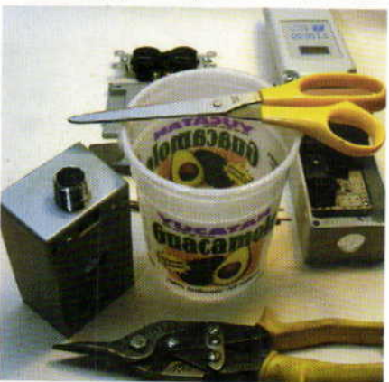
With ordinary shears or aviation snips, cut a plastic or non-metallic material for a spacer.
