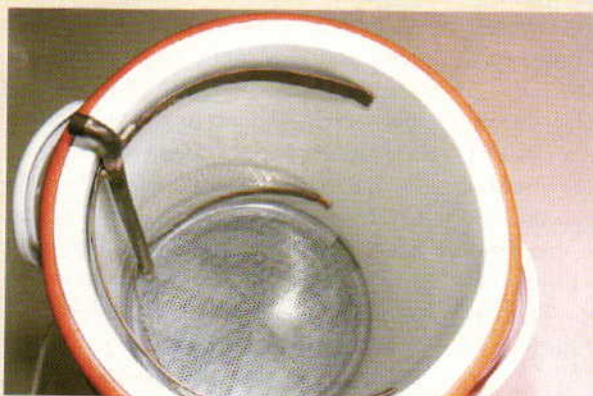
The combination mash and lauter tun is a time and space saver. Add heat to the tun and you have a RIMS.
