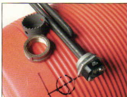
Using the appropriate size hole saw, cut a hole in your cooler for your heating element.
