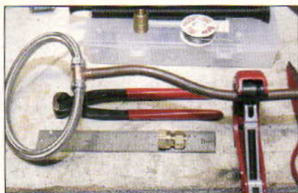
Use a tube bender to curve the copper tubing to the bottom of the tun and cut to fit.
