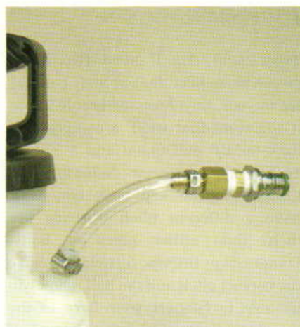
Be sure to remember your hose clamps to ensure a tight seal.
