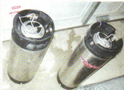
Two kegs full of sanitizing solution. The keg lids hang in the solution from their latches.
