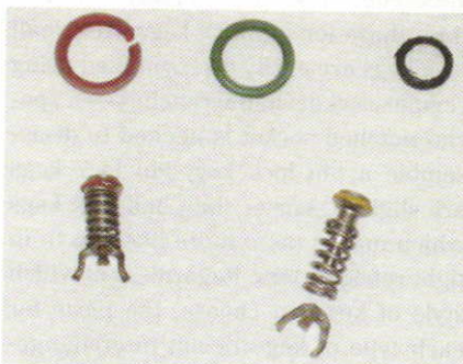
Broken and dry-rotted o-rings need to be replaced, as do broken poppets.
