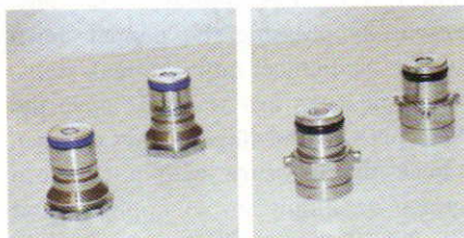
Left: ball lock posts from a Pepsi keg. Right: pin lock posts from a Coke keg.
