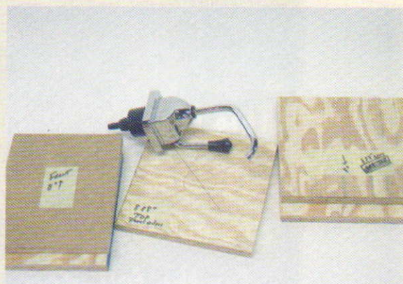
A few pieces of plywood, and a hand pump is all you need to make your authentic beer engine for some "real ale."
