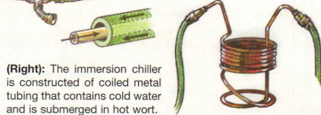
(Left): The counter-flow chiller runs hot wort through a tube that is within a tube of cold flowing water.
