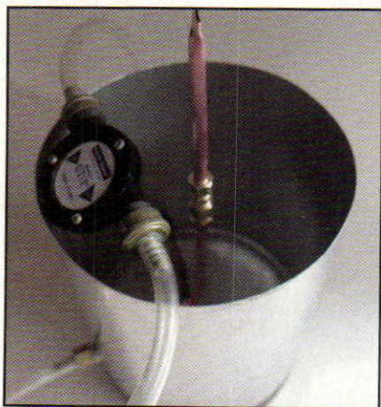
Utilize a drill-powered pump in order to power your bottle sprayer and your fermenter cleaner.
