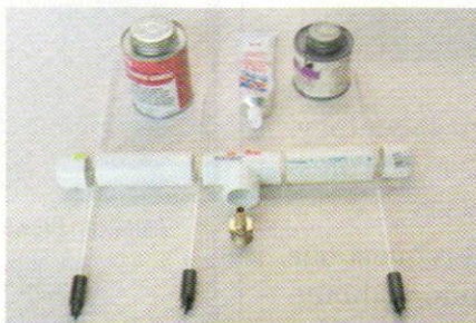
Assembling the manifold requires cutting and drilling this CPVC water pipe and securing its connection with glue.
