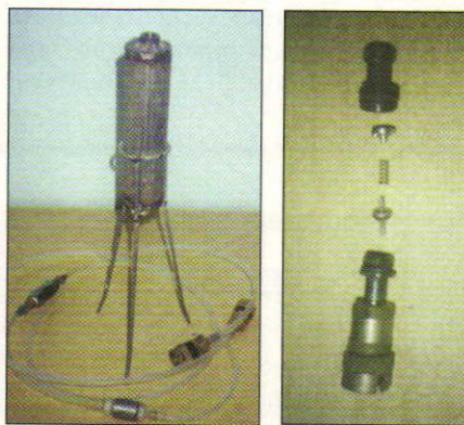
(left): The homemade filter pushes beer through diatomaceous earth (DE). (right): Components of the pressure valve.
