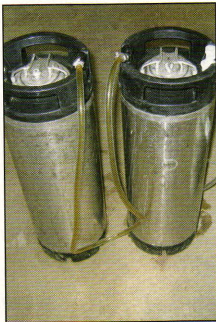
With a jumper line attached to the “beer out” posts of two Corny kegs, beer can be transferred without contact with air.
