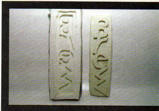
(top): Pour the silicone over your clay and let it cure over night. Here you can see the dried mold. (bottom): You can then pour in the casting resin and let it cure. On the right is the casted, unpainted mold.
