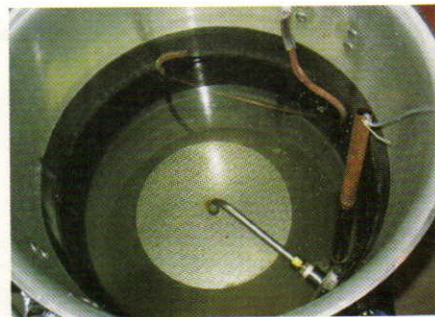
This is the mash tun with a heat sensor and slotted manifold.
