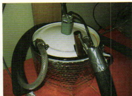
Here is the heat exchanger with a stirrer in the lid. The sensor protrudes from the front.
