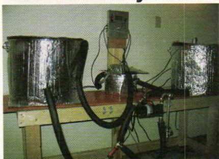
This is Mark's mash tun, heating element, lauter tun, pump and controller.
