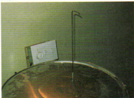
The stir sticks are constructed of coat hangers that are bent and cut to size.
