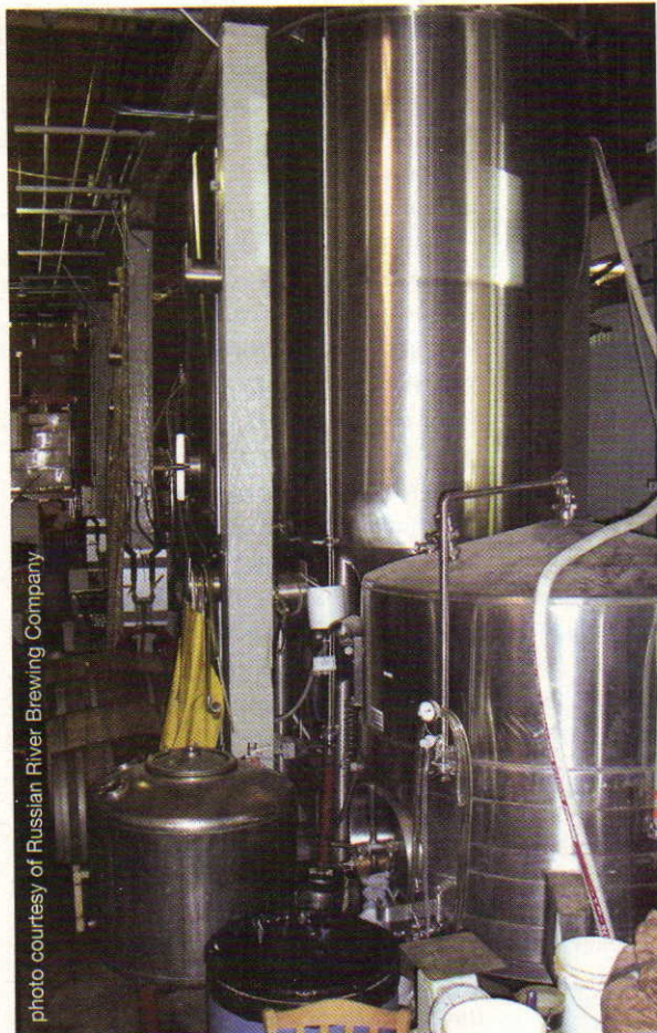
Closed, upright fermenters at Russian River and an open, shallow fermenter at Ommegang. Most homebrewers use closed fermenters (buckets or carboys), but many are experimenting with open fermentation. Open, shallow fermentation allows for more air contact with the yeast, faster heat dispersal and easier top cropping.
