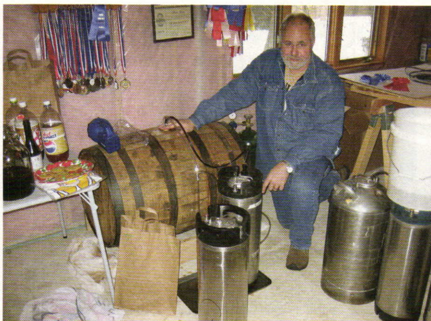
You will need to brew at least 60 gallons (227 L) of beer to fill a 53-gallon (201-L) bourbon barrel. Beer will evaporate through the joints over time and the barrel will need to be topped up. Once you're finished, the beer can be pushed by CO 2 pressure (as shown in the photo above) into Cornelius kegs.
