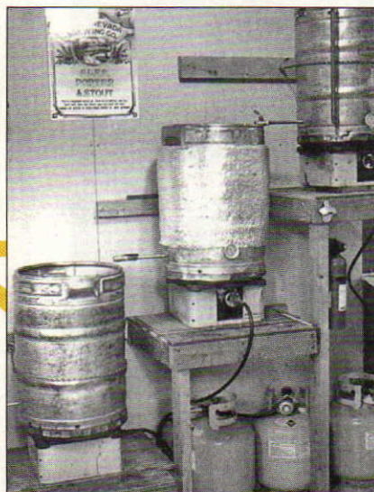
John's original three-tier system. The top two vessels have ball valves and the water or wort flows through vinyl tubing.
