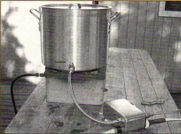
Here is Palmer's 8-gallon (30-L) aluminum pot on top of his propane burner, connected to his plate chiller. He drilled the hole for the ball valve and installed a weldless fitting.
