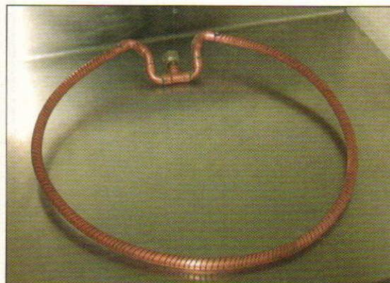
A close-up of Rob's pick-up ring (manifold). He cut each of these slots individually with a hacksaw.
