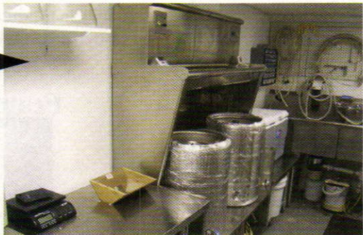
The system has two Sabco kettles, one being the brew kettle, the other the hot liquor tun. Each has a 4,500-watt, 240-V electric heating element.
