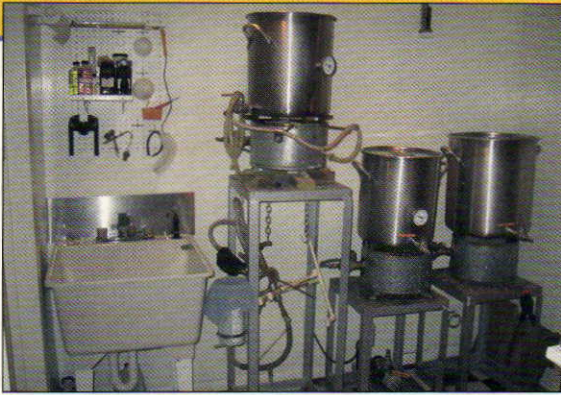
A look at Beck's hot-side equipment. From left to right, the hot liquor tank, mash tun and kettle. His system is located in his basement and is fired with natural gas.
