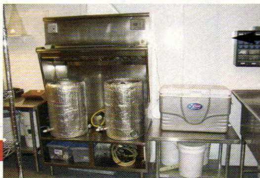
The system has two Sabco kettles, one being the brew kettle, the other the hot liquor tun. Each has a 4,500-watt, 240-V electric heating element.
