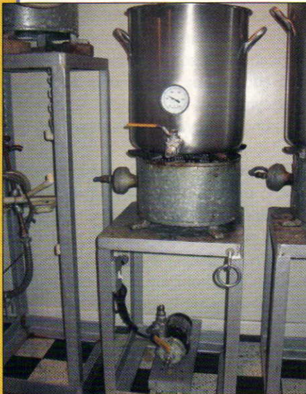
A close up of Beck's mash tun with the pump mounted below it. The ball valves on the mash tun and pump are fitted with quick disconnects.
