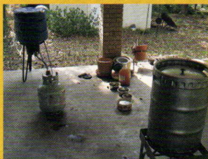
I usually mash in a 10-gallon (38-L) pot, shown here with its insulating jacket on. A keggie is my hot liquor tank (HLT).
