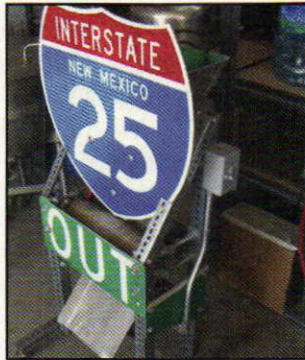
TWO ROLLER MILL – The motorized two roller mill was inspired by a salvaged highway sign. The hopper holds 30 pounds (13.5 kg) of grain and the 4" diameter rollers are adjustable for control of the crush.
