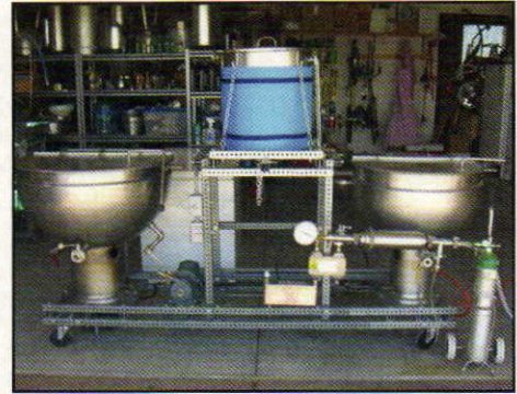
FULL RIG – The rolling brewery rig consists of two steam kettles: a 60-gallon (228-L) HLT and a 40-gallon (152-L) kettle/mash cooker. The 35-gallon (133-L) mash/lauter tun pivots to dump its spent grain and doubles as a whirlpool. Both gravity and a stainless steel centrifugal pump are utilized to transfer liquid.
