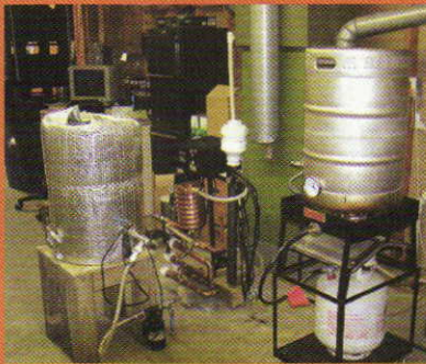
The heat exchanger & controller setup is in the middle of the shot, mashtun on the left (a Sanke wrapped in R19 insulation), boiler on the right.
