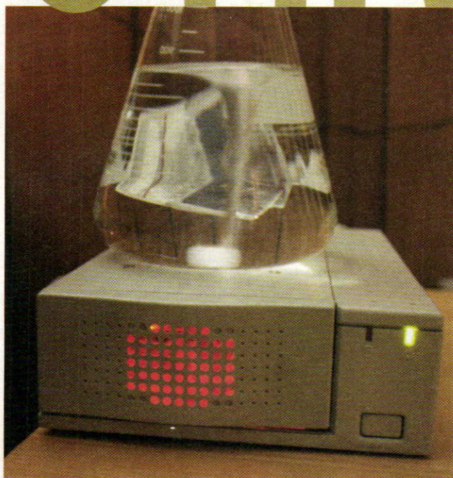
"I'm sorry, I can't let you underpitch, Dave." With a stir plate, you can raise more cells in your yeast starter.
