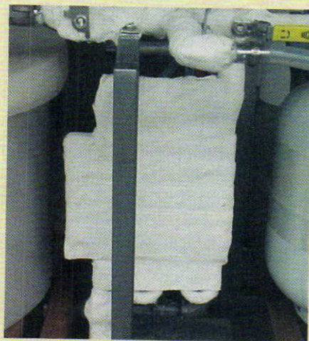
The heaters are similar to a heat exchanger. I use an aluminum plate which has 4 passes of wort flowing through 1/2" copper tubing.
