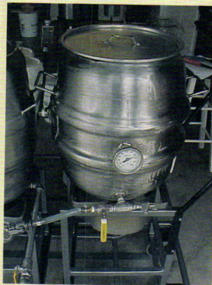
The brew kettle has a stainless steel check valve and downstream is a valve to slow the sparge, which normally takes 30 minutes.
