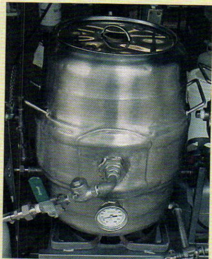
This is the hot liquor tank. There is a small sampling valve tee'd the other way in case I need extra water for the boil.
