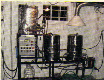
My HERMS brew system consists of three converted kegs, a magnetic pump, and is powered by three 240 volt heating elements.
