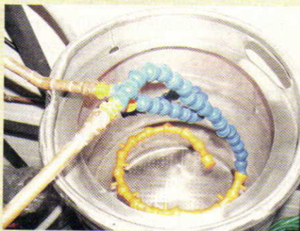
This is the inside view of the mash tun showing the hinged false bottom and the sparge arm.
