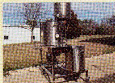
Randy's 3-tier system uses three stainless steel, aluminum-clad, 15-gallon vessels and a Shirron plate chiller.
