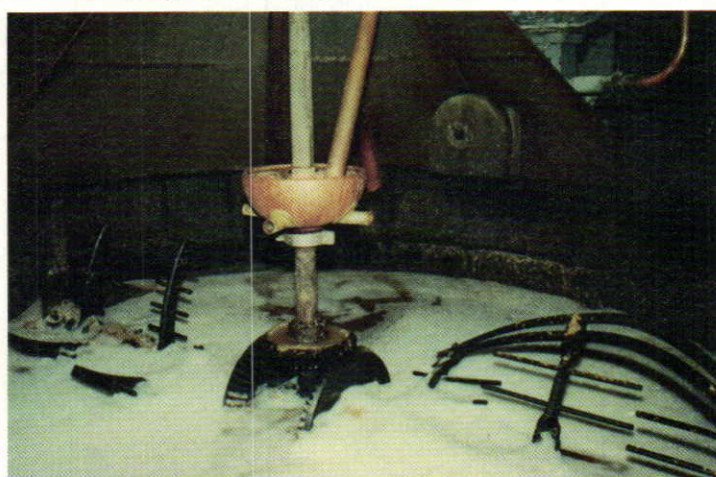
The apparatus in a turbid mash tun stirs the mash and doubles as a manifold. Earlier versions of turbid mashing employed a wicker basket.
