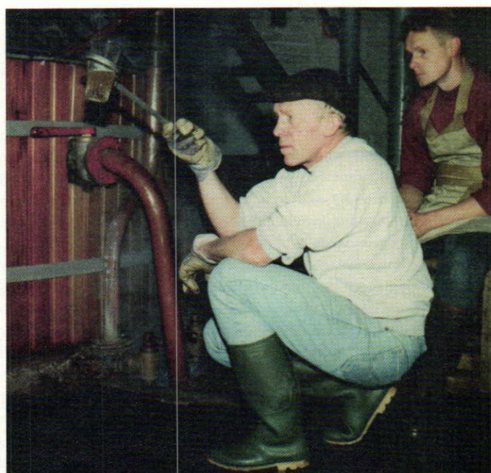
J.P. Van Roy examines the cloudy wort pulled from a turbid mash. The starches in this wort will slowly feed the souring microorganisms in a lambic.
