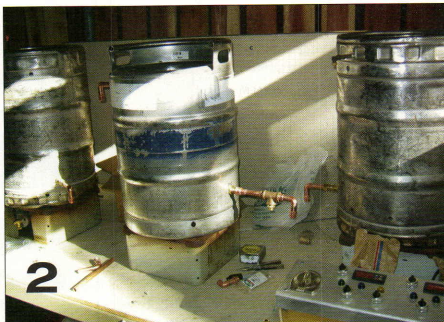
Figure 2: Here is the brewstand in progress. The hot liquor tank (HLT) is on the right, behind the control panel. The silicone tubing will connect onto the copper fittings coming out of the kegs, and go through the table to the pump and valves below.
