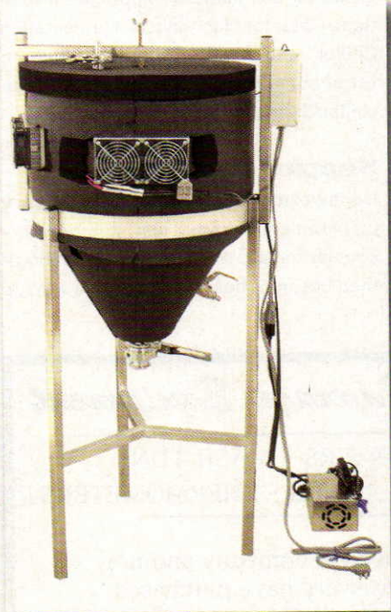
Maintaining both warm and cool fermentation temperatures is made easier with a glycol-jacketed conical fermenter.
