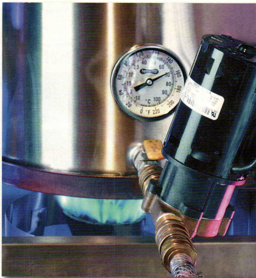
A lit propane burner with the proper oxygen to fuel mix will exhibit a stable blue flame with just a touch of yellow at the base.
