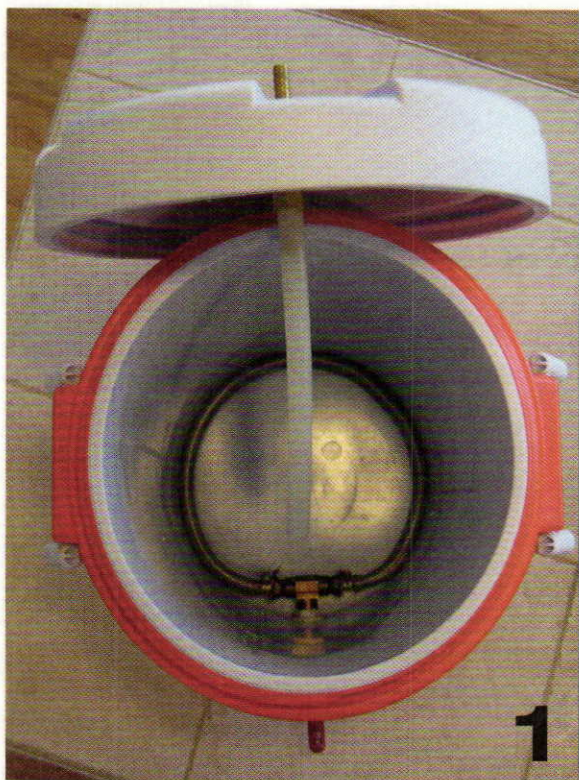
1. Mash/Lauter Tun (MLT): A \frac{3}{8} " ball valve is fitted to the outside of the cooler. Inside, stainless steel braid (from a washing machine connector) connects to both ends of a \frac{3}{8} " T-connector. The lid is fitted with \frac{3}{8} " fittings.
